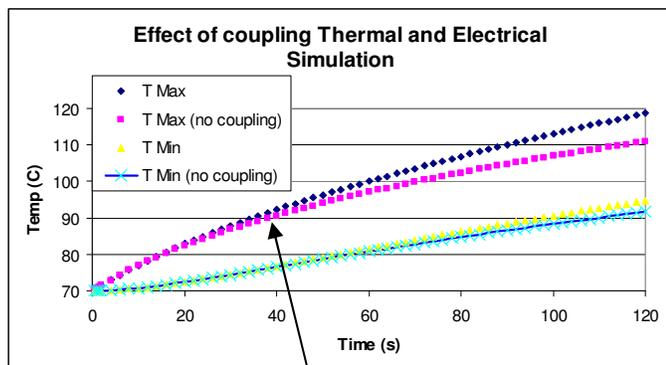
As temperature increases the electrical resistance increases, causing higher heat dissipation.
